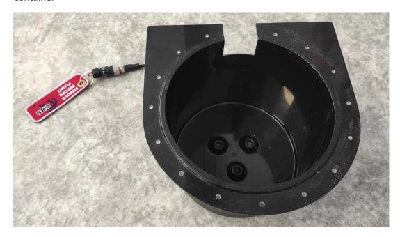
2) We recommend to attach the canister by 3 bolts, make holes according to the picture below. It is good to cover pins for pyroactuators by sticker during drilling. It is needed to consider the effect of pyrotechnic device during activation. Consider the installation of the sensitive electro devices just under the bottom of the canister. Canister should be placed on rigid plate.
