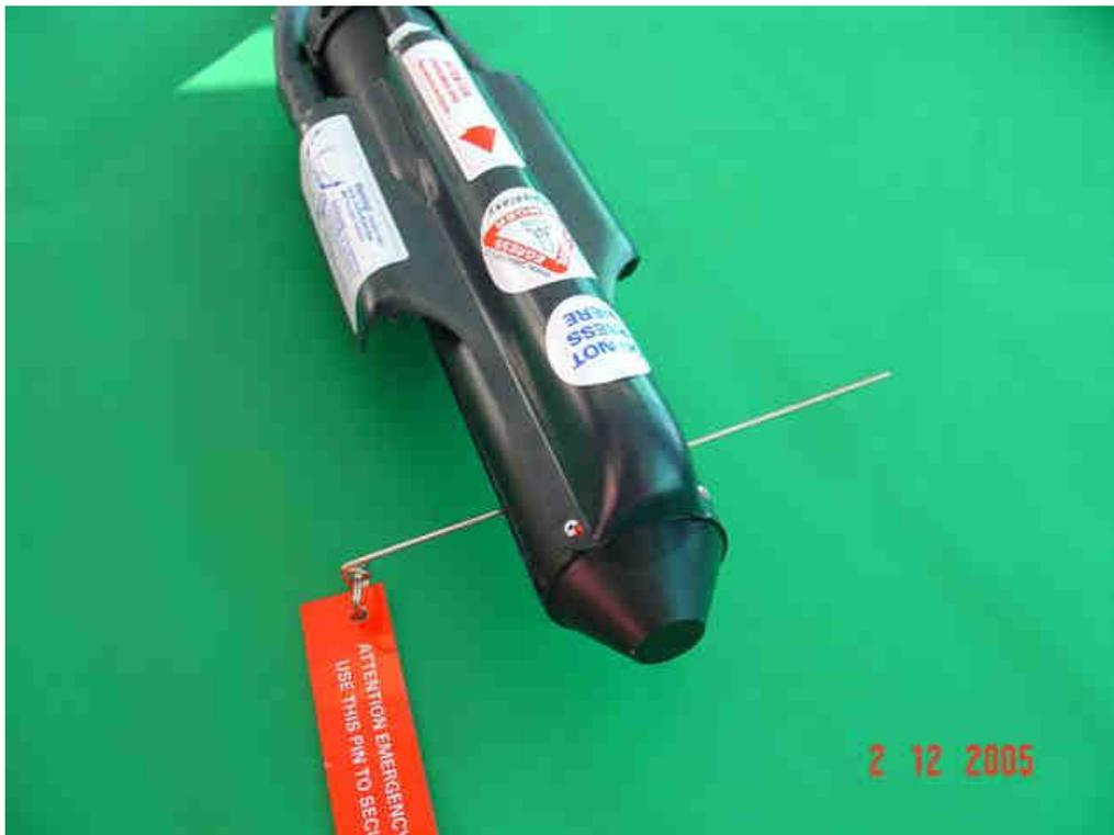
5. Bend the tip of the pin to prevent it from being removed from the rocket.
