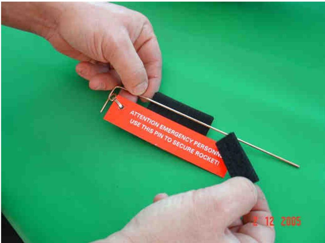
3. Place the end of the pin into the hole inside the silver colored launch tube. This hole has a RED outline and is about half-way up the exposed portion of the rocket and can be seen from either side of the rocket. The pin **MUST** go completely through the rocket motor and out the other side, or the rocket is not secure!.
