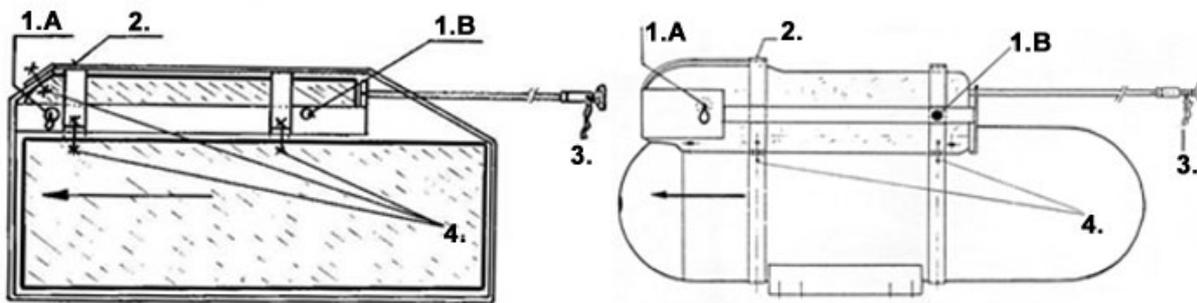
1. Transport saf1. Safety **A-** of steel wire diameter 2 mm, **B M5 bolt**.
