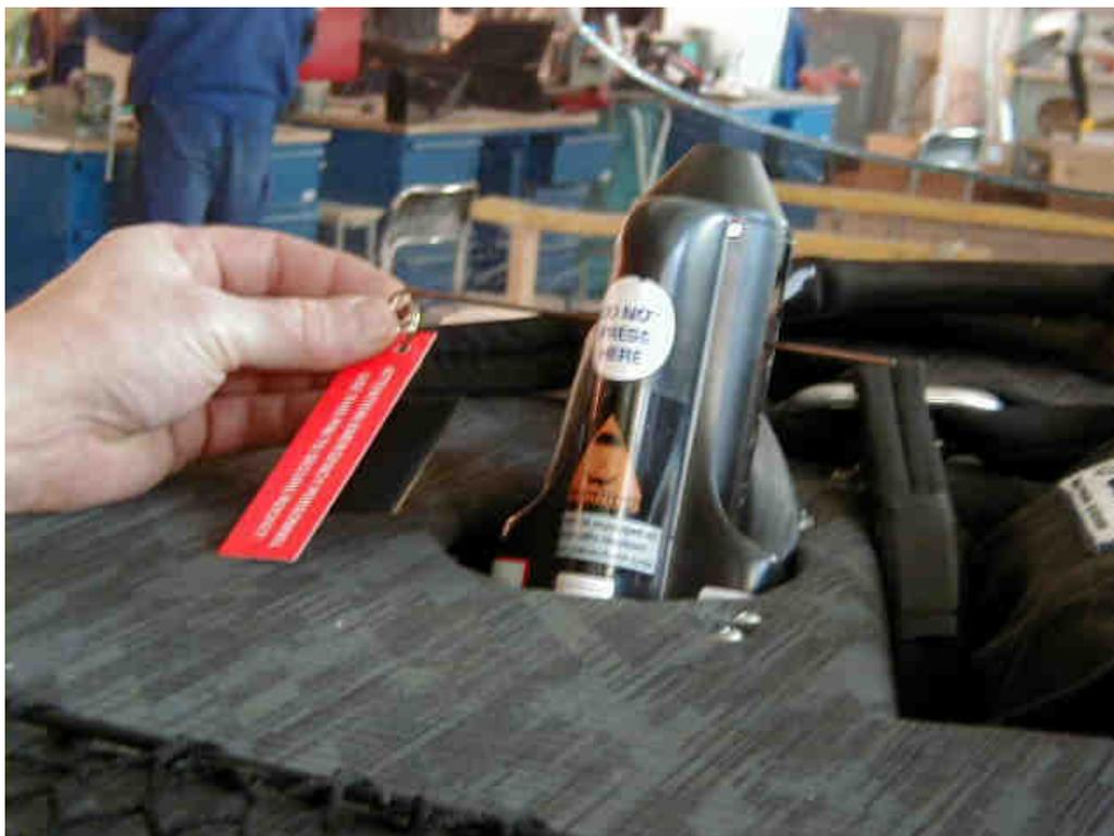
4. The pin can be inserted from either direction but must go completely through the rocket engine and housing.
